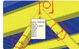
Example of change management – Using redline markings, colors, and tooltips to illustrate design changes in a 3D model
